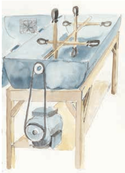
The thrashing machine has a small motor to rotate manomin.
